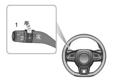
With the START/STOP Switch in the ON/READY position and the headlamps on, rotate the fog lamp switch to position I to turn on the rear fog lamps. The rear fog lamp indicator illuminates in the instrument pack when the rear fog lamps are on.
