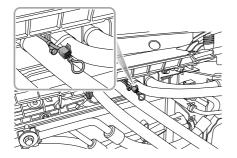
Pull the release cable handle, remove the connector plug whilst maintaining tension on the cable this will release the locking device.
