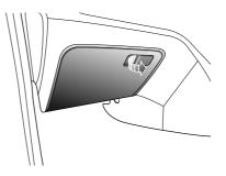
To open the glove box, pull the handle on the glove box cover (as indicated by the arrow).
