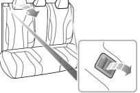
To increase the luggage space, the rear seat backrest can be folded fully forward. When folding the backrest completely, firstly insert the rear seat belt buckle into the corresponding slot, then fully lower (or remove) all head restraints, pull the respective control lever at the top of the seat backrest upwards and fold the seat backrest forward.
