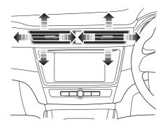
Slide the button in the centre of the louvres completely to the left or right to open or close the vent. Toggle it up and down, left and right to adjust the air direction.
