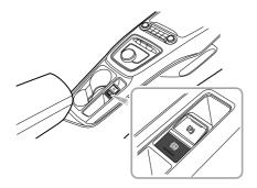
With the driver's seat belt fastened, the door closed and the power system operating, press the auto hold switch to switch the auto hold function from Off to the Standby state.
