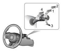
The rear wiper and washer will only operate when the START/STOP Switch is in the ON/READY position. Rotate the rear window wiper switch to your desired selection:
