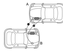
Ensure the START/STOP Switch is turned off and switch off ALL electrical equipment of BOTH vehicles, then follow the instructions below:
