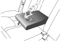
Fold forward to open the rear armrest. There are cup holders at the front end of the rear armrest.
