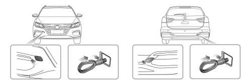
Your car is equipped with 2 towing eyes (located at the front and the rear of the vehicle), which are used for fitting the towing hook in the tool kit. The tool kit is placed beneath the loadspace floor.
