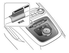
The driver can manually select three driving modes by operating the MODE switch on the centre console: Eco Mode, Normal Mode and Sport Mode.
