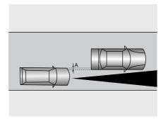
When driving behind a vehicle that is only partially overlapping your vehicle, 'A' in the graphic, the adaptive cruise control system may be unable to detect anything.
