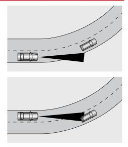
When turning at an intersection or following a vehicle into, or out of a curve, the adaptive cruise control system may be unable to detect the vehicle ahead, even if it is in the same lane, it is possible the system may detect a vehicle in another lane.
