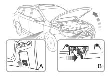
From the inside of the vehicle, pull the bonnet release handle (Figure A).
