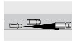
If the vehicle ahead changes lanes, but does not drive into the lane completely, the adaptive cruise control system may be unable to detect the vehicle.
