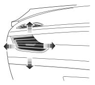
Slide the button in the centre of the louvres completely to the left or right to open or close the vent. Toggle it up and down, left and right to adjust the air direction.
