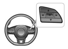
Press the UP/DOWN/LEFT/RIGHT button in the RH steering wheel multifunction switch pack, this will access and display the general information options.
