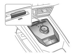
The driver can select three energy regeneration levels by operating the KERS switch :
