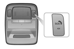
The emergency services call (eCall) system will perform a self-test when the vehicle power system/ignition is turned ON. During a Self-Test the emergency services call (eCall) LED status indicator on the SOS button will flash quickly until completion. The LED status indicator will illuminate permenantly if no system faults are present. The LED status indicator will be extinguished or flash slowly if a
