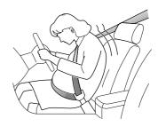
The diagonal section of the seat belt should pass across the chest as normal, the lap section of the belt should pass below the belly, low and snug on the hip bones. NEVER position the belt on or above the belly.
