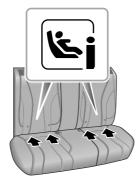
3 To fasten the Top tether strap of the child restraint system, route the tether strap under the head restraint and attach to the anchorage hook being careful not to twist the strap. If not using ISOFIX lower anchorages, using the seatbelt, complete the installation in line with the child restraint manufactures instructions. Note: When using seat mounting, universally approved child restraint systems, Top tether must be used.
